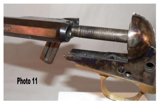
(Make sure you stick the arbor in the arbor hole and not the bore!) Now, rotate the bottom of the barrel down until it contacts the frame. The barrel should set flush with the frame or just a few thousands up or down from the frame. Photo 12 shows our Pietta barrel mates perfectly with the frame.
