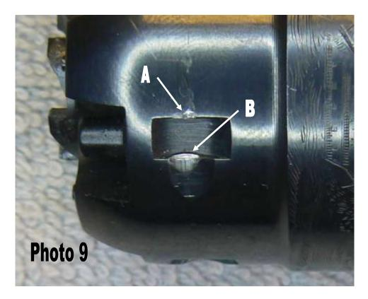
What is happening is that rather than locking bank vault tight, our cylinder is simply getting a wedgie from the bolt. Fitting the bolt is the main part of our tune up. With the cylinder off, Photo 10 shows the frame is slightly miscast.
