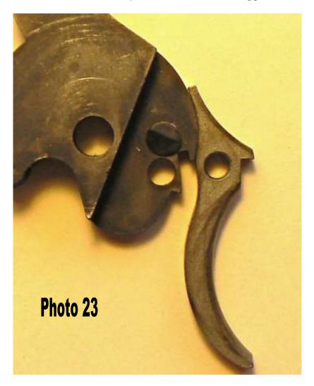
The top of the trigger above the trigger screw hole slides along the front of the hammer until the trigger tip drops into the half cock or full cock notches. On a lot of guns, the back of the trigger or front of the hammer is very roughly ground and you can feel grittiness while cocking the hammer as the trigger drags over the front of the hammer. On our project gun, the front of the hammer and back of the trigger is smooth and need little, if any, polishing.
