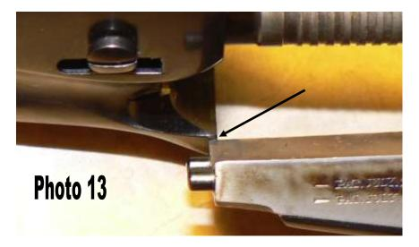
The Uberti arbor is far to short and the barrel sets well behind the front of the frame. There are exceptions to all rules, but in general Piettas have poorly fitted bolts and good arbor fit. Ubertis have properly fitted bolts and poor arbor fit. (We will tune an Uberti in a future article and fix a poorly fitted arbor.) Now we will begin final disassembly of our Pietta and look for obvious internal problems.
