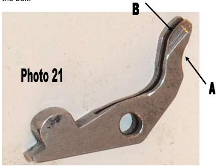
Although the Pietta bolt head is typically too wide, the bolt body is very nicely made and very smooth compared to many other Colt clones. It has a very nice bevel on the end of the bolt leg that rides on the hammer cam. See above Photo 21 (B).
