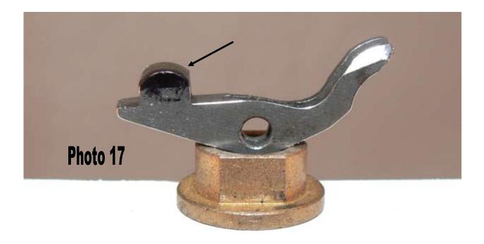
We do not want to remove material below the marked area. Photo 18 (A) shows the burr we identified when cycling the hammer.
