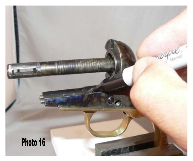
Now, remove the main spring, the trigger guard, the bolt/sear spring, the trigger, the bolt, and finally, the hammer and hand (some people refer to it as a pawl). Now that the bolt is out, be careful not to rub off the black color until we get around to fitting the bolt. Photo 17 shows the bolt and the area in black that is ABOVE the bolt window in the frame.
