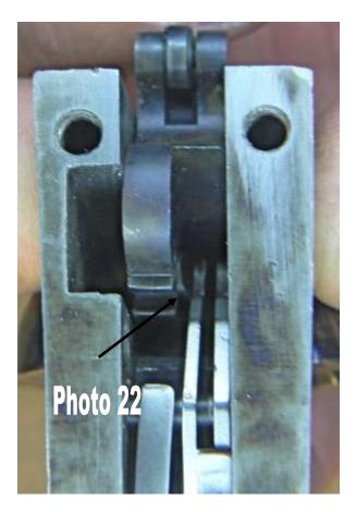
When the hammer is all the way down, the leg of the bolt snaps back over the top of the hammer cam and the process begins again for the next shot. (In Photo 22, the bent leg
