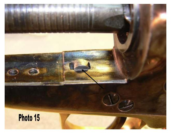
If we narrow the entire head of the bolt it will fit the cylinder notches, but it will fit too loosely in the frame window and the cylinder will have excessive side-to-side play. Just to make sure what area needs to be narrowed, take a Sharpie and color the side of the bolt as shown in photo 16. (Only color the side shown, we will not take material from the other side.)
