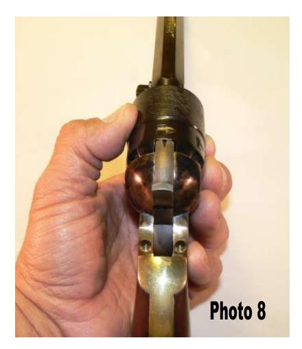
Do this for each chamber. On this gun, its mate, and several other Piettas I handled at EOT, most of them would unlock on at least one chamber. So, even though most Piettas (we are talking about the newer Colt style Piettas made in the last five years or so) feel like they are locked up "bank-vault" tight, they are not and that is the primary problem we will address in our tune-up.
