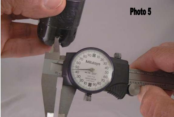
As we had previously diagnosed, the bolt appeared too wide and was peening the bolt notches. Our bolt measures .157". Photo 6.
