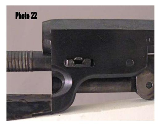
When the gun is shot, the wedge will loosen a little more and the wedge will go a little further into the barrel. As long as the wedge is tight, it doesn't matter if the tip of the wedge spring is past the edge of the barrel. The primary purpose of the spring isn't to lock the wedge into the barrel. It's primary purpose is to catch on the wedge screw and keep the wedge from falling out of the barrel when it is pulled loose to remove the barrel for cleaning.
