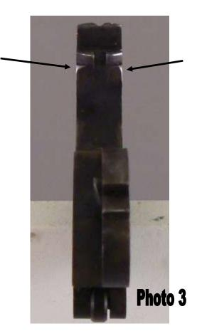
It isn't necessary (or possible on some guns) to completely remove all side-to-side hammer contact. What we want is a smooth transition in the event the hammer happens to rub on the frame while shooting. Once the hammer moves smoothly in the frame, we will move on to the most critical part of our tune-up--fitting the cylinder bolt to the cylinder.
